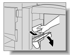
9 Clockwise turn the misfeedclearing dial in the folding section. Feed out into the lower output tray the paper that could not be fed out in step 8, and then pull out the paper.
